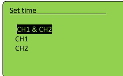
Now you can select the decimal with the keys ◀ or ▶ and with the keys ▲ or ▼ you can set the time to the desired value. Confirm with OK (✓) to return to the main menu.
