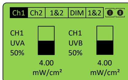
Stop an irradiation by pressing ✓ for at least 2 seconds.
