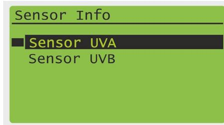
Display information about the sensor. If no sensor is connected, this menu item is not displayed.
