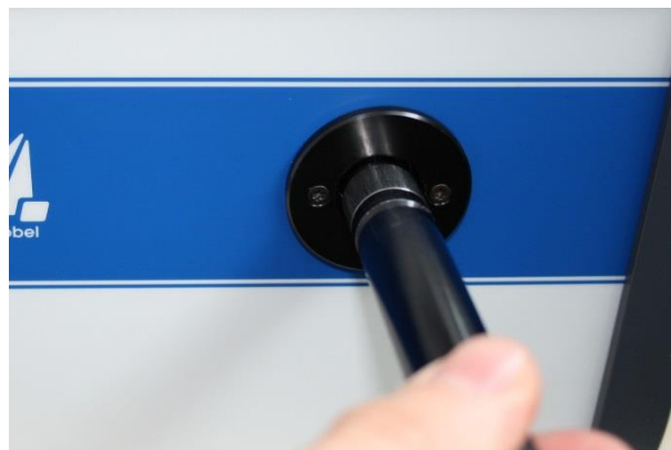
Figure 2: Inserting the light conductor
